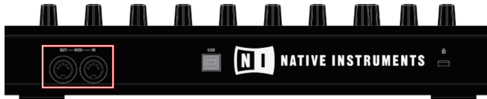
The back side of the MASCHINE Hardware with the MIDI In port
